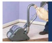
TIP: If starting with a 24 or 40 grit belt, never skip a grade in the sanding process, you must use all grits available before finishing with a 120 grit belt.
